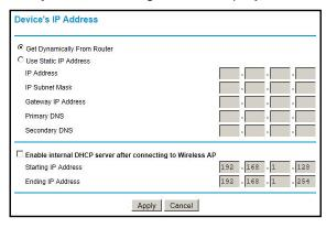
This screen shows whether the Internet adapter is set to get its IP address dynamically from the router (this is the most common setting), or is set with a static IP address.
